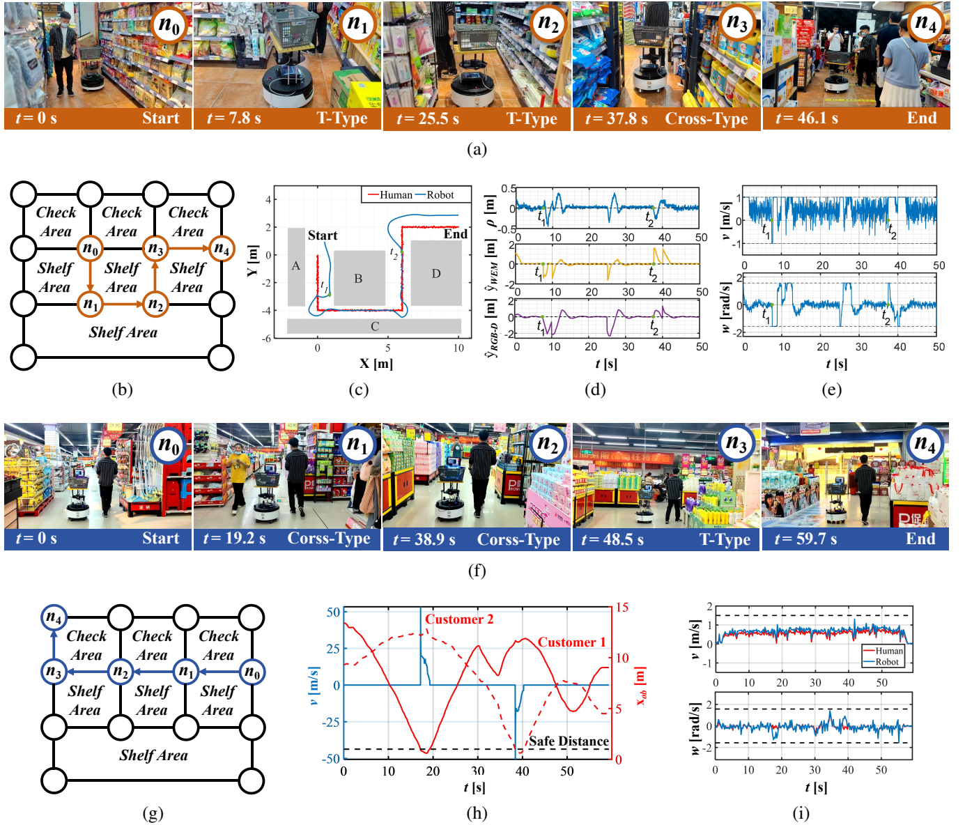
Fig. 7. Experimental results of intersection-aware following in supermarket environments. (a) The snapshot of the intersection-aware following experiment. (b) The path node. (c) Trajectories of human target and SSR. (d) The SSR's motion state. (e) The SSR's control input. (f) Snapshots of the social avoidance experiment. (g) The map with the path nodes. (h) The output of the obstacle avoidance control. (i) The control input of the SSR and human target.
